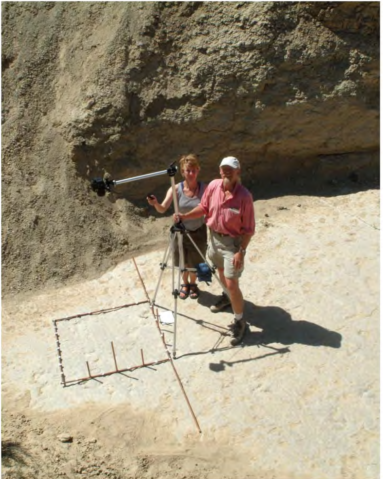
A fixed grid of varying height was used as an early method of providing x,y, and z control at the Red Gulch Dinosaur Tracksite in Wyoming.
